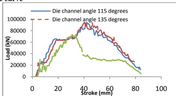
**Fig.3.** Load-stroke comparison at different die angles during ECAE
